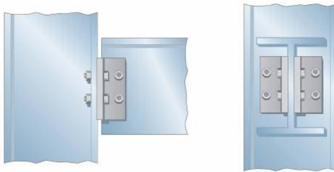
typical “pin-supported” connection (metal)
