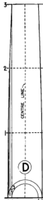
D METHOD FOR ENTASIS abcd ARE BOTTOM & TOP DIAMETERS RESPECTIVELY. DESCRIBE SEMICIRCLES ON THESE & AT c DRECT PERPENDICULAR CUTTING LARGER ONE IN 3. DIVIDE SEGMENT a 3 & HEIGHT OF COLUMN INTO ANY NUMBER OF EQUAL PARTS - SAY 3 - & NUMBER BOTH 1/23 FROM a. THRO' POINTS 1/23 IN SEGMENT ERECT PERPENDICULARS CUTTING CORRESPONDING DIVISIONS OF THE HEIGHT THRO' THE POINTS THUS OBTAINED DRAW CURVE
