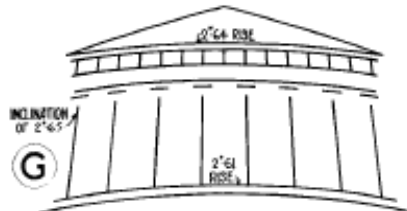
D METHOD FOR ENTASIS abcd ARE BOTTOM & TOP DIAMETERS RESPECTIVELY. DESCRIBE SEMICIRCLES ON THESE & AT c DRECT PERPENDICULAR CUTTING LARGER ONE IN 3. DIVIDE SEGMENT a 3 & HEIGHT OF COLUMN INTO ANY NUMBER OF EQUAL PARTS - SAY 3 - & NUMBER BOTH 1/23 FROM a. THRO' POINTS 1/23 IN SEGMENT ERECT PERPENDICULARS CUTTING CORRESPONDING DIVISIONS OF THE HEIGHT THRO' THE POINTS THUS OBTAINED DRAW CURVE
