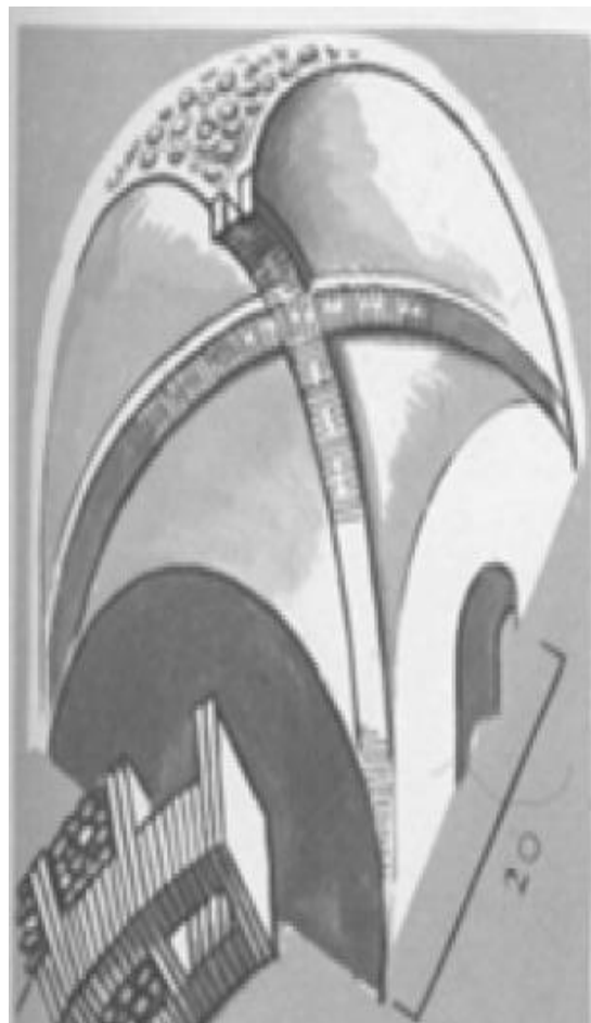
Cross-vault built of brick ribs and filled in with concrete Villa Sette Bassi, near Rome, C. A.D. 123-134
