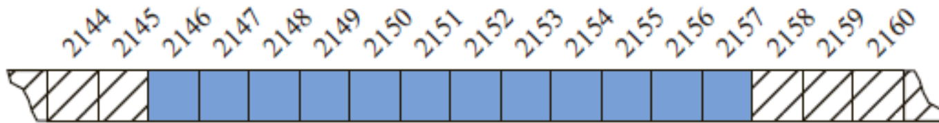
Figure 7.2: An array of 12 cells, allocated in memory locations 2146 through 2157.
