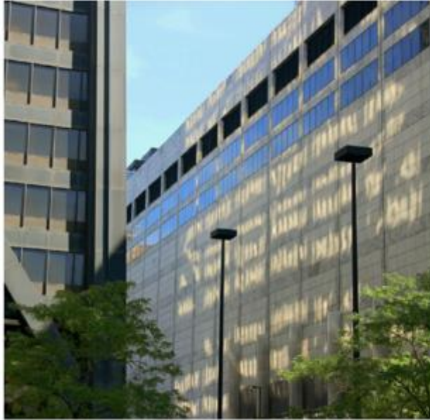
Figure 9.2f Glass facades without exterior shading devices reflect much of the sun. The bright spots on the north side of this building are a result of reflections from the building on the left.
