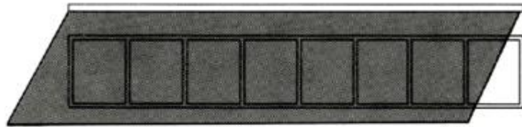
Figure 9.6c Wide strip windows make efficient use of the horizontal overhang.
