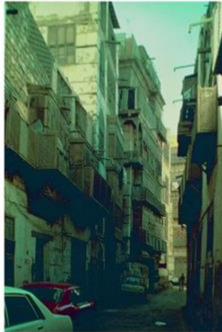
Figure 11.1c Multistory buildings facing narrow streets create desirable shade in very hot climates, as here in Jidda, Saudi Arabia. (Photograph by Richard Millman.)
