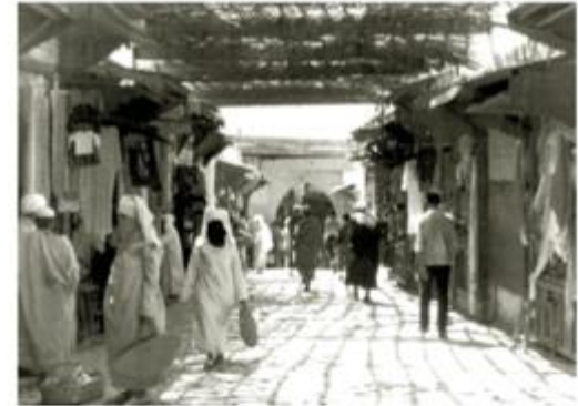
Figure 11.1d The shading structure over this Moroccan street blocks much of the sun but still allows air and daylight to filter through. (Courtesy of the Moroccan National Tourist Office.)
